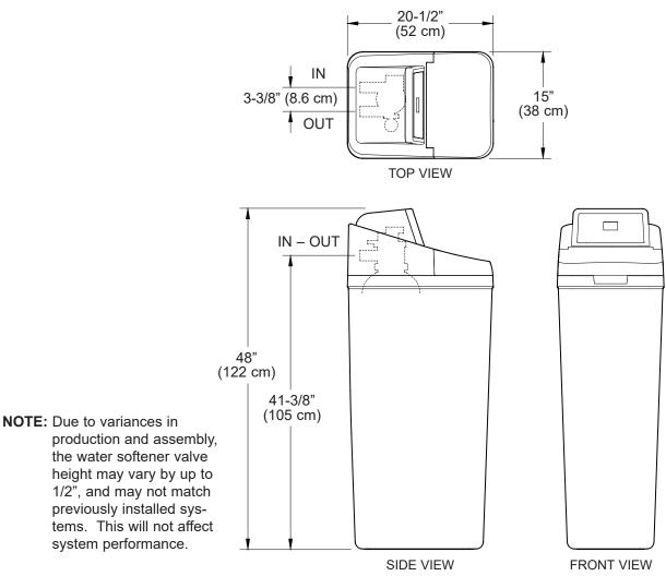
the water softener valve height may vary by up to 1/2", and may not match previously installed systems. This will not affect system performance.
