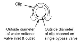
NOTE: Be sure all 3 tabs of the clip go through the matching holes on the water softener valve inlet or outlet, and fully into the channel on the single bypass valve.
